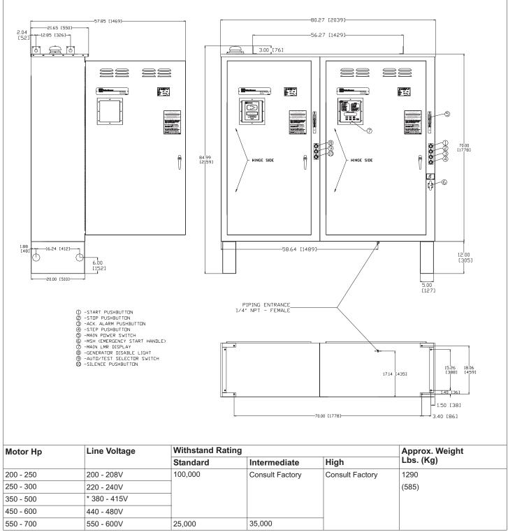
\* Coils available: 380V-50Hz, 380V-60Hz, 415V-50Hz, 415V-60Hz.
