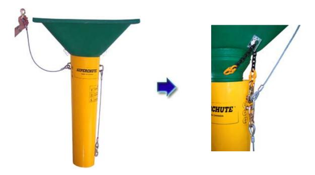
**WARNING!** Do not use the funnel to support the tremie sections hanging below. It is not strong enough. Use the cable assemblies or U-bolts of the uppermost tremie section to support the weight of the tremie sections hanging below.
